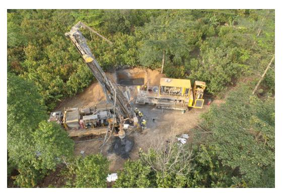
Figure 10-17: Reverse Circulation Drill (Newcore, 2021)
