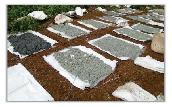
Figure 10-24: Drying Wet RC Samples (Newcore, 2017)
