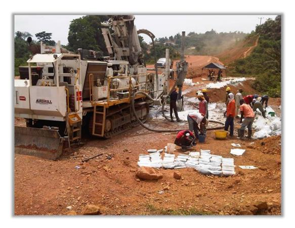
Figure 10-1: Reverse Circulation Drill (Newcore, 2012)
