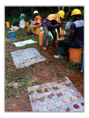
Figure 10-19: RC Chip Logging (Newcore, 2017)
