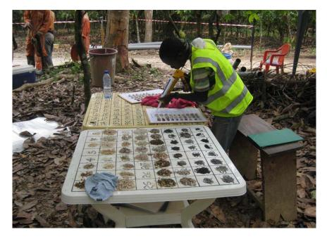
Figure 10-20: Chip Board Preparation (Newcore, 2017)
