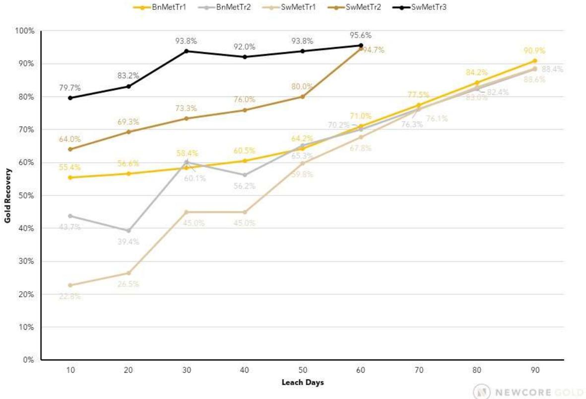
The column tests are aimed at simulating the response to leaching of the sample with the emphasis on establishing the gold dissolution characteristics (rate and extent), reagent consumption, and the degree of slumping within the ore bed. All samples showed amenability to heap leaching, with recoveries averaging 91.7% after 60 to 90 days.
